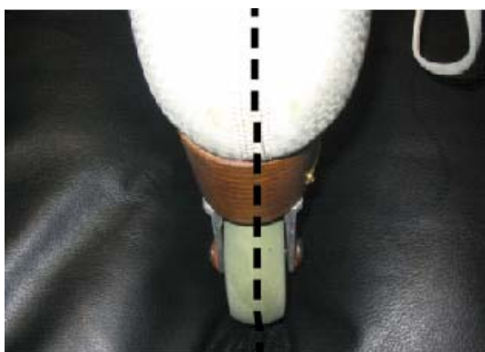
Figure 2. Heel alignment centreline.
